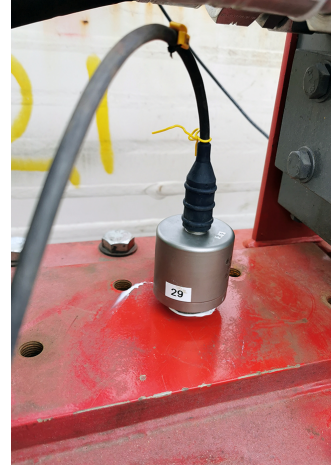
(b) a_2 on the actuator housing.
